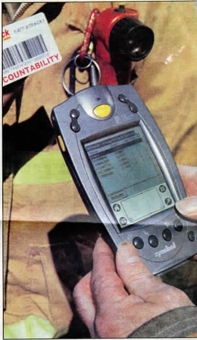
The XTrack's hand-held device works on a magnetic antenna and chip, and information logged into the system can be uploaded onto a PC, which creates secure reports and audits the trail of fire scene activities from the web site ( www.XTrack.com ). Also on the site is a collection of firefighters' recipes from around the world, an honor roll and photographs, which is accessible to the public. (Cassie D. Lavertue photo)
