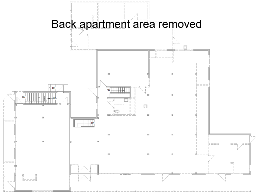
1 LEVEL 1 - DEMOLITION PLAN Scale: 1/8" = 1'-0"
