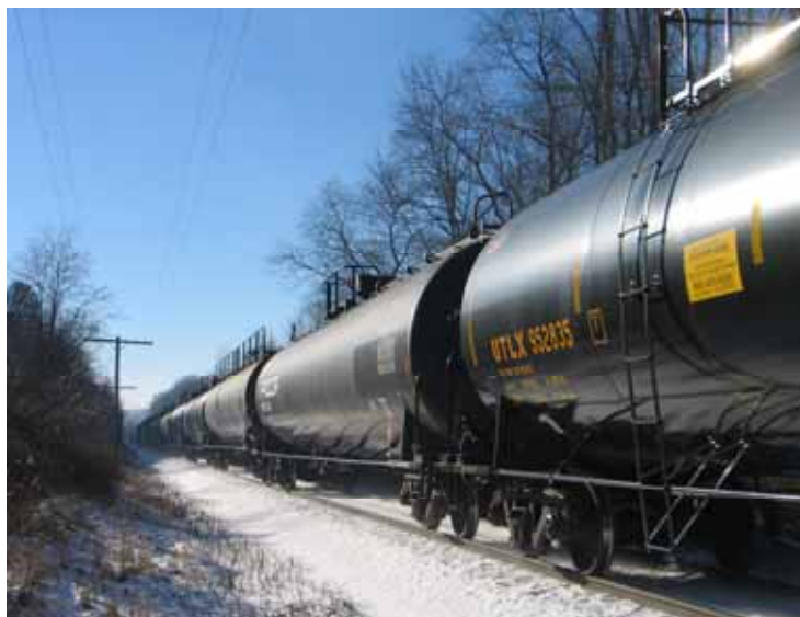
Freight train consisting of Liquefied Petroleum Gas (LPG) tank cars rolls through Cornish on the New England Central Railroad.
